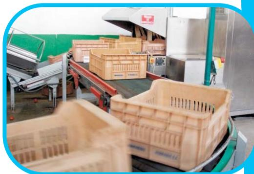
The machinery consists of a washing-tank (2,200 – 3,000 litres) and a rinsing-tank with a closed circuit of water. During the washing of the boxes a filter keeps any particles out (dust, any remains of the product, etc), so the water is always free from particles in suspension and can therefore be re-used every day to wash the boxes.
